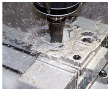
Large hole drilling using high-torque specs Machining details Hole diameter: ø40mm Material: Carbon steel
