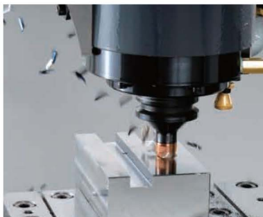
Grooving using standard specs Machining details Cutting amount: 150cc/min Material: Carbon steel (for ø16 end mill)
